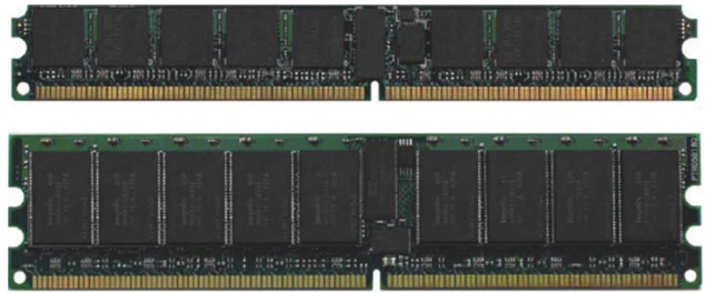
Figure 6 The very-low-profile DIMMs are essentially the same as the standard DIMMs but at 60% of the height.
